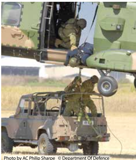
Perentie being hitched under helicopter during an external lift trial.
