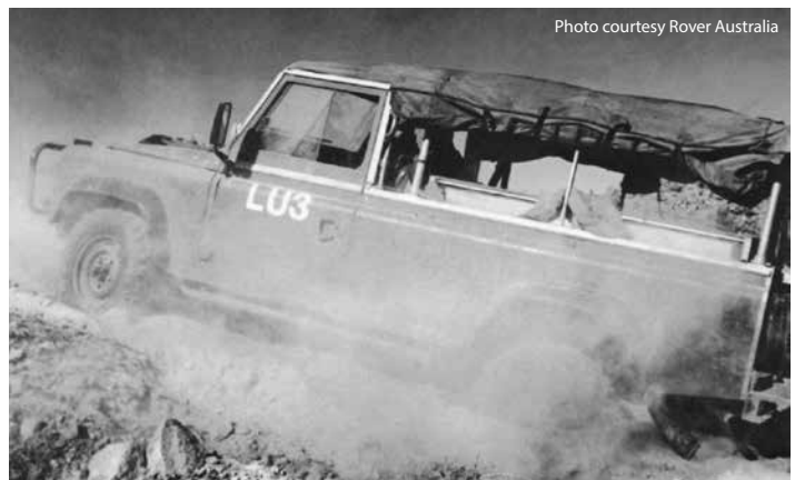
One of the 4x4 Trials vehicles undergoing accelerated testing at Army's Trials and Proving Ground at Monegeetta, near Melbourne.
