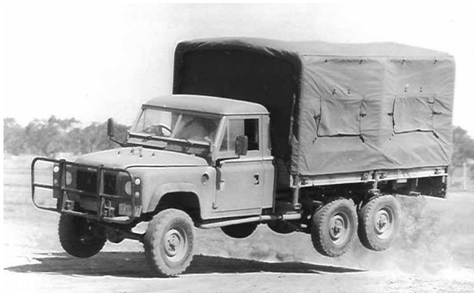
Land Rover put its vehicles through extreme durability testing even before they went to the Army trials. This is the Sandringham being tested after the chassis modifications.
