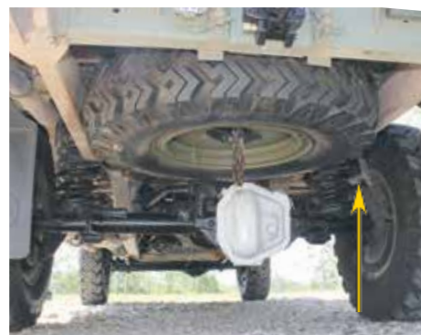
Perentie's rear chassis is unique. Note white diff cover and convoy light (arrowed).
